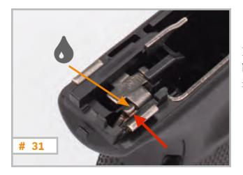
EDC Pro Tip: Push the rear end of the trigger bar inward (toward the left side) to open the right rear corner to place the drop of oil.
